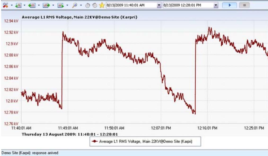
From here, it is possible to select the Zoom out ratio. Therefore an **X3 ratio** yields the three time larger interval as below
